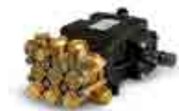
Pompa professionale in linea (a bielle) con testata in ottone e tre pistoni in ceramica. In line professional pump (with connecting rods), brass head, and three ceramic pistons.
